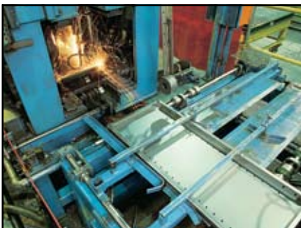
Automated welding of Hi-Performance shelves.
